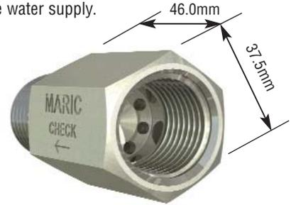
**Non-Return Feature.** The maintenance free design of the Maric valve uses the flow control rubber as the flexible sealing component in the non-return mechanism. The flexing of the control rubber under normal operating conditions prevents scale build-up on the rubbers surface, which ensures a reliable seal, even after extended periods of no reverse pressure.
